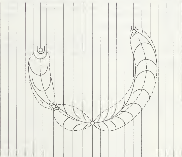
Figure 27: (Top) Nematic and (centre) smectic liquid crystals viewed through microscopes equipped with crossed polarizers. (Bottom) Spatial variation of the director, causing the threadlike image seen in the photograph at top.
